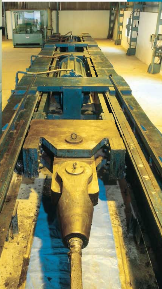
Testing facility ranging from 100 kN for wire to 10000 kN for rope
