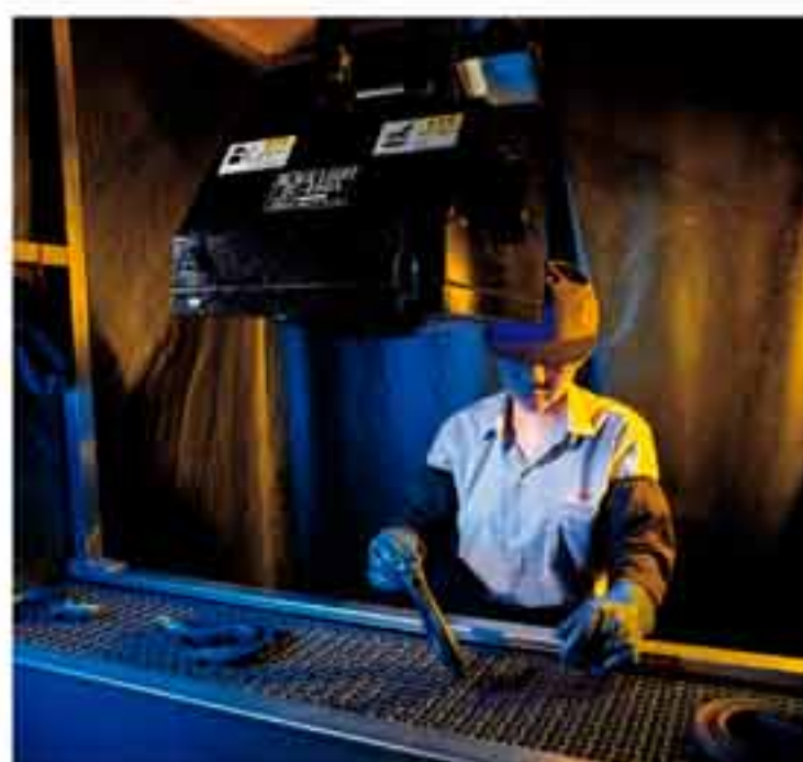
Magnaflux Crack Detection
