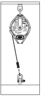
The anchorage point on the protected load must be directly below the overhead anchorage point. Attaching the safety line directly below the overhead anchorage, to the central point of the load will help to minimise the amount of swing and dangerous movement when a fall is stopped. Attaching the load off centre will cause the load to rotate, which could cause further hazards or in extreme cases, damage to the supporting safety line.
