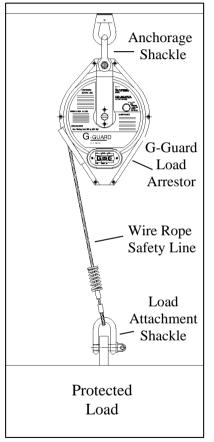
The wire rope safety line is spring tensioned so that it extracts and retracts from the unit, ensuring that there is no slack rope. This enables the load to move freely while keeping the potential fall distance to a minimum.
